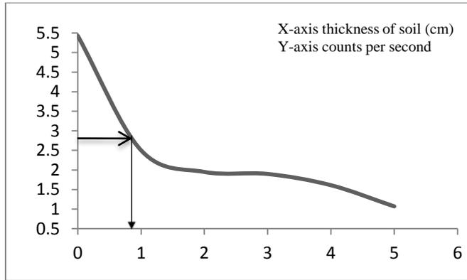
Fig. (1) Attenuation graph for Cs-137 Gamma Source (Loikaw)
